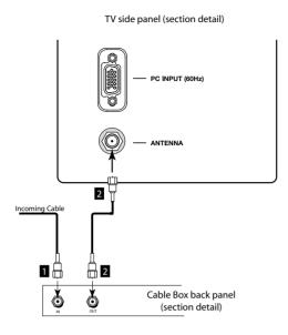
Figure 3. Connecting the cable box.
